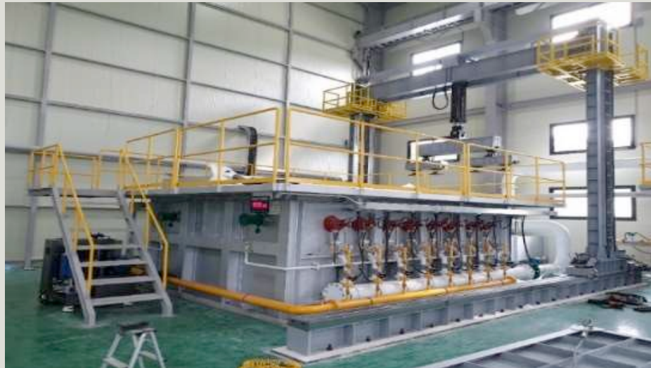
(Fire resistance test equipment for horizontal members)
